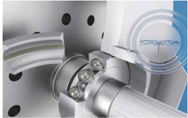
Shaft voltage discharge in an EV motor bearing
